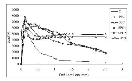
Figure 5. Load-deflection curves in fracture tests.
