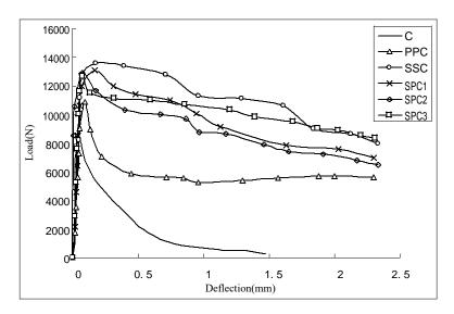
Figure 4. Load-deflection curves in flexural toughness tests.
