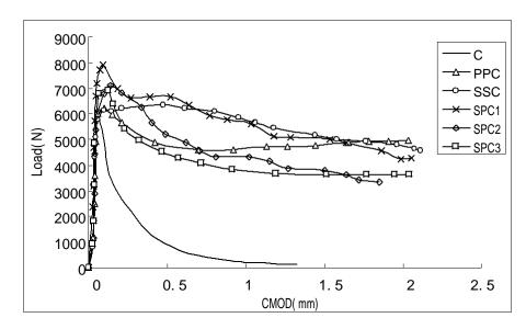
Figure 6. Load-CMOD curves in fracture tests.
