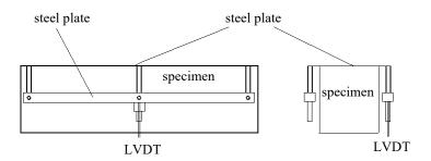
Figure 1. Flexural toughness test.
