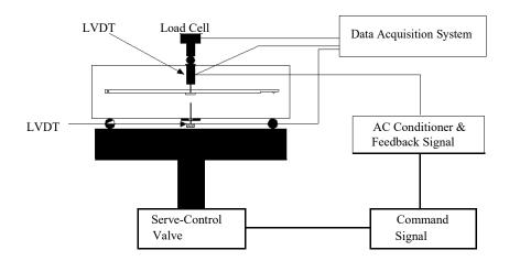
Figure 3. Schematics of flexural test setup.
