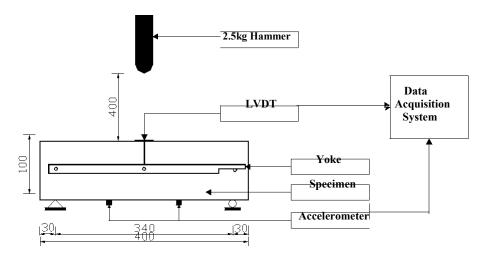
Figure 2. Drop weight flexural impact equipment.
