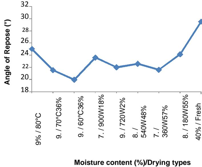
**Figure 4.** Effect of moisture content/ drying types on angle of repose of laurel berry.
