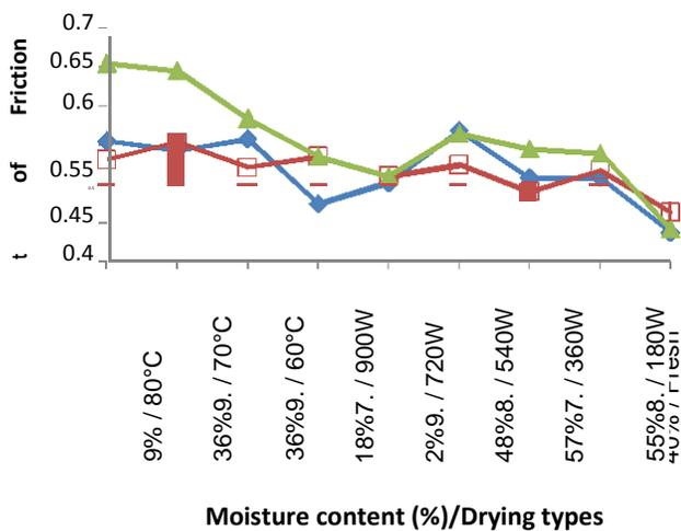
**Figure 3.** Effect of moisture content on coefficient of friction of laurel berry with chrome steel (♦); galvanized steel (■); plywood (▲).
