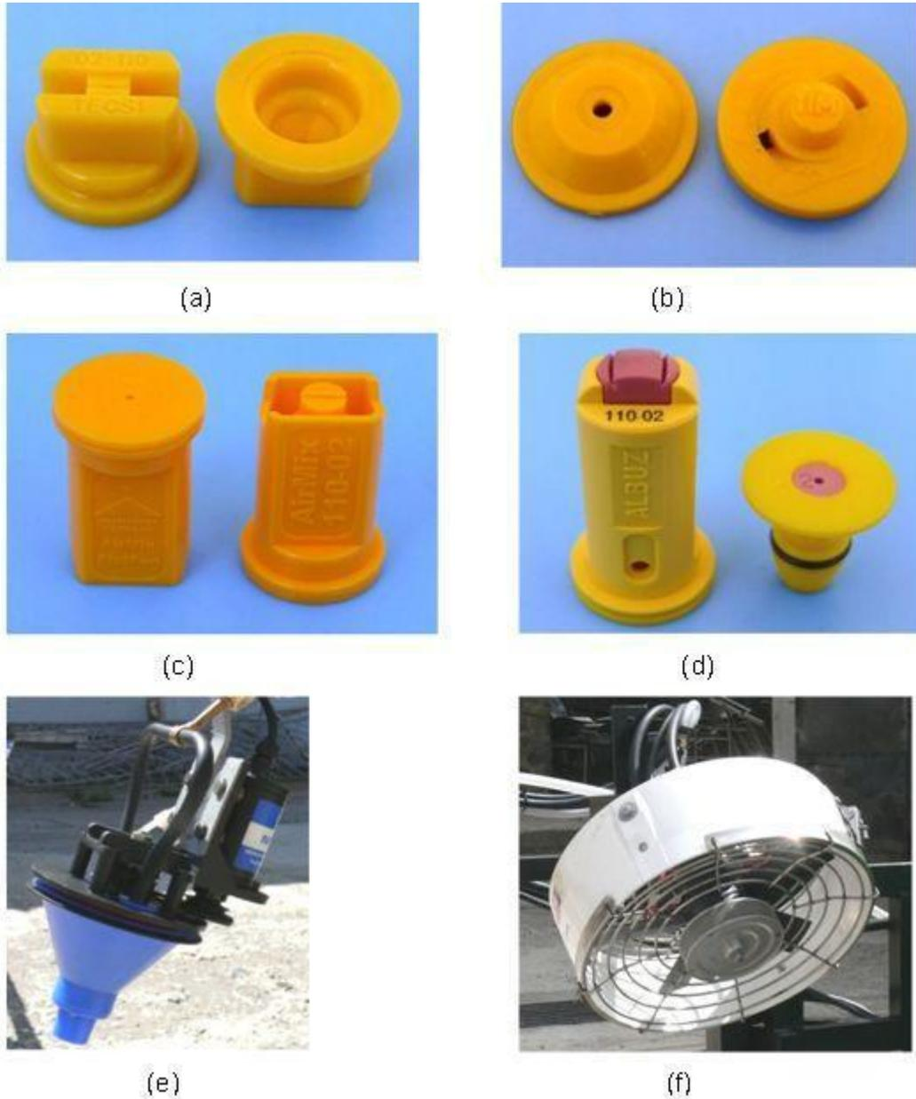
**Figure 1.** Spray nozzles (a) standard flat fan nozzle, FF, Tecsi SRL 11002 (b) hollow cone nozzle, HC, Tim Ø1.0 (c) air induction nozzle, AI, Agrotop 11002 (d) twin jet with air induction nozzle, TJ, Albus AVI TWIN 11002 (e) spinning disc nozzle, SD, Micromax®, CDA (f) air assisted rotary atomizer, RA, Proptec™ rotary atomizer.
