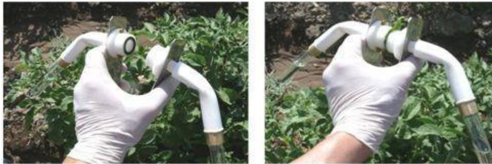
**Figure 3.** Washing the leaf samples with the dual-side washer.
