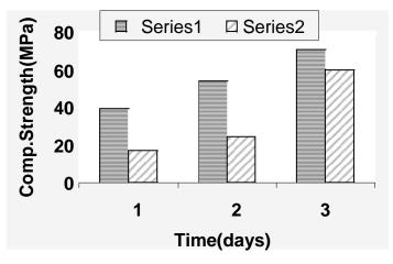
Figure 9. Variation of compressive strength with time. Series1-OPC, Series2-Blended cement
