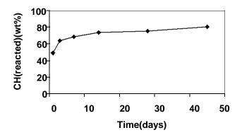
**Figure 7.** Amount of calcium hydroxide reacted with BLA in a paste at different time as determined by DSC technique
