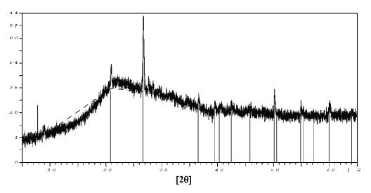
Figure 3. X-ray diffraction pattern of Bamboo leaf ash.
