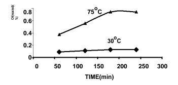
**Figure 4.** Amount of calcium hydroxide reacted at different time with BLA in suspension at different temperatures
