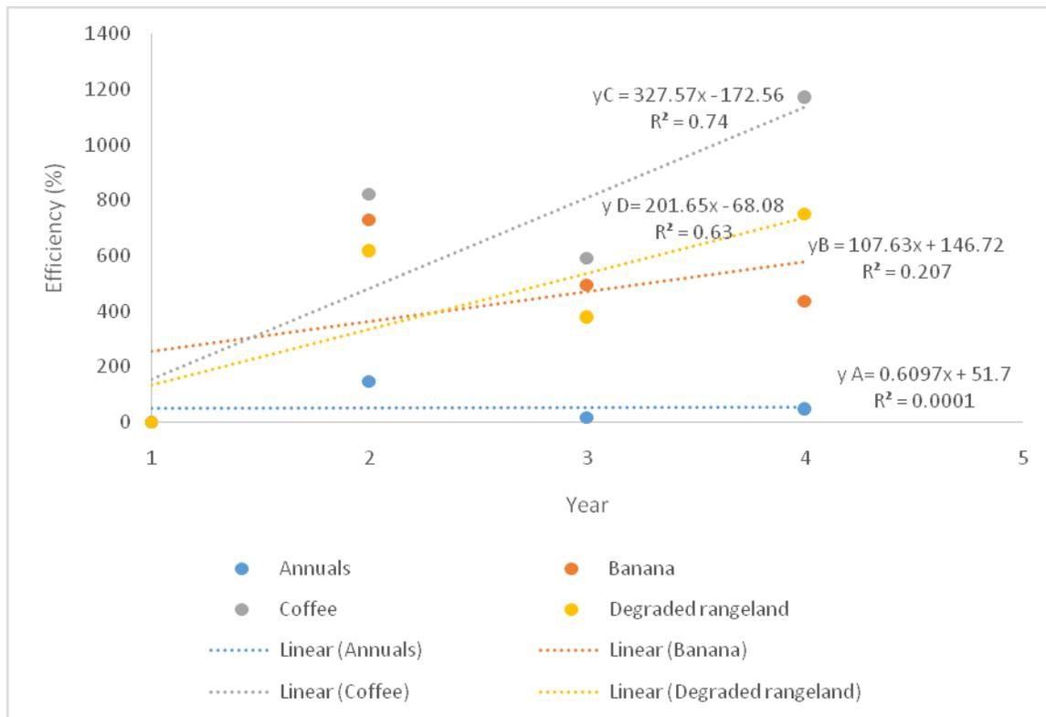
**Figure 4.** Efficiency of contour bunds in reducing runoff from selected agricultural land-use in Bukoora sub-catchment-Lake Victoria basin.
