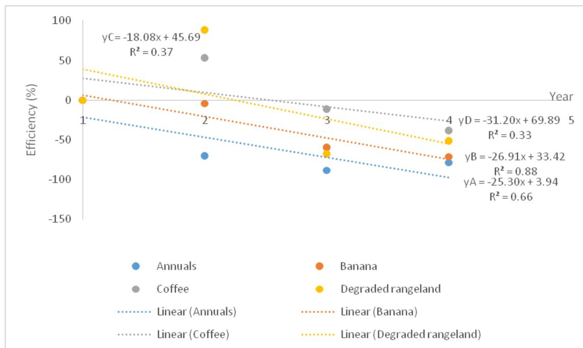
**Figure 3.** Efficiency of contour bunds in reducing soil loss from selected agricultural land-use in Bukoora sub-catchment-Lake Victoria basin.
