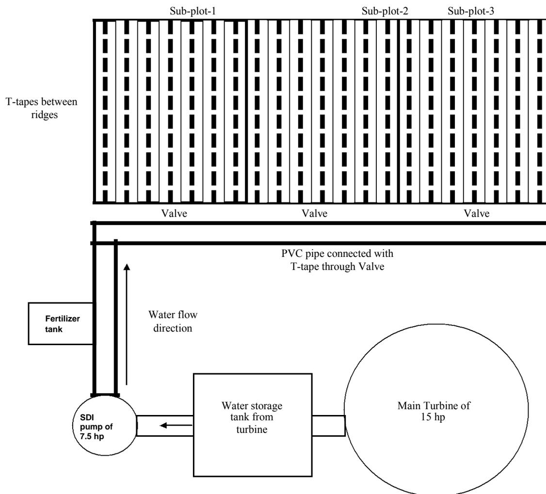
**Figure 1.** Layout of T-tapes system for sugar cane.
