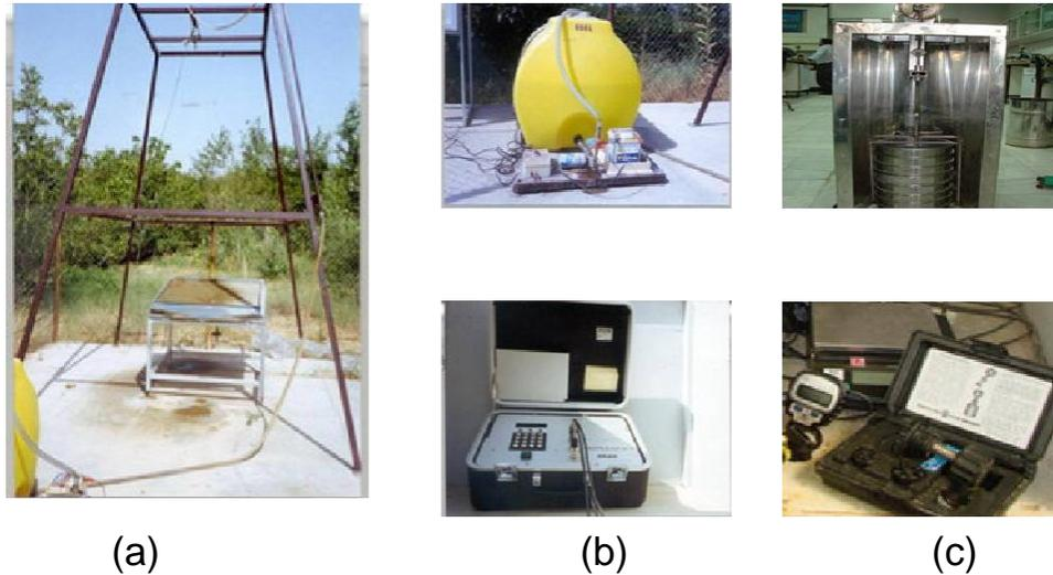
**Figure 2.** The research institute of forests and rangelands of Iran (IRIFR) tilting flume and simulated rainfall facility consisting of: (a) steel frame with oscillating nozzle and tilting flume, (b) water container with water pump (up) and electronic control system (down) and (c) wet sieving apparatus (up) torvane (down).
