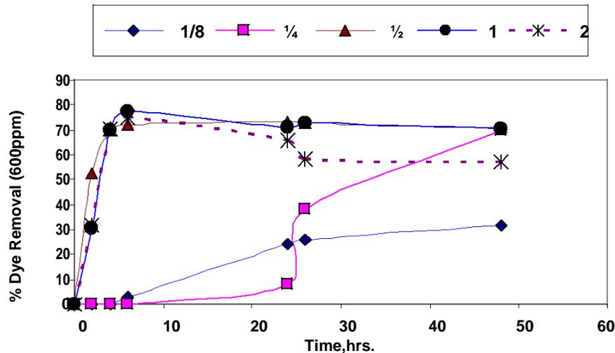
**Figure 2.** Effect of aeration on removing of dis-azo dye using fungal strain 20 (after addition 600 ppm dye).
