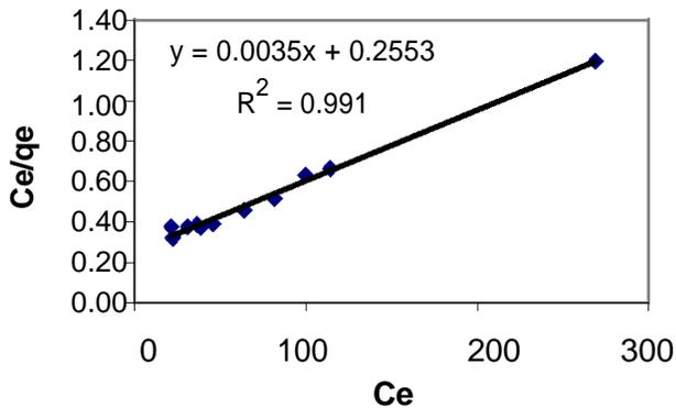
**Figure 6.** The linearized Langmuir adsorption isotherm of direct dye by fungal biomass at pH 5.5 and T = 28-30°C.
