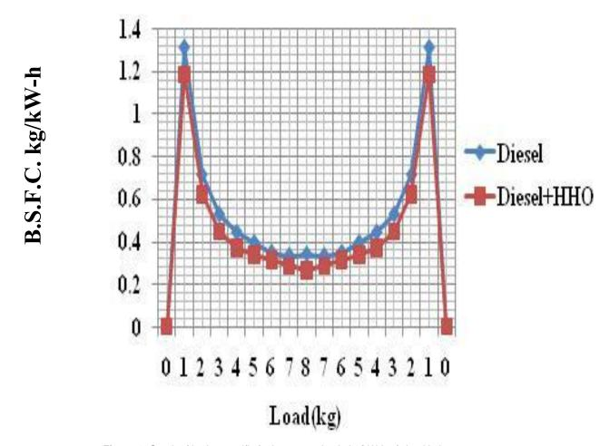
Figure 6. Graph of brake specific fuel consumption in kg/kW-h v/s load in kg.
