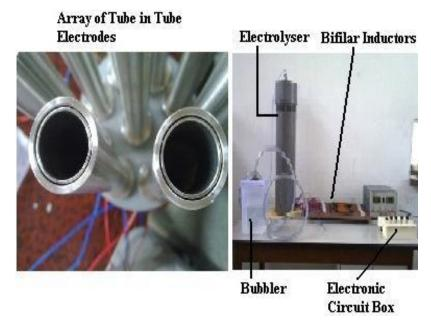
**Figure 3.** Arrangements of electrodes in second method of electrolyser and other components.
