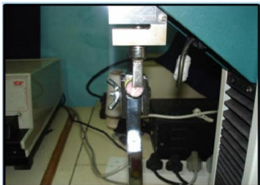
**Figure 3.** Specimen mounted on custom made jig, load applied at a cross head speed of 0.5 mm/min using a blade parallel to the dentin surface until the specimen shears.
