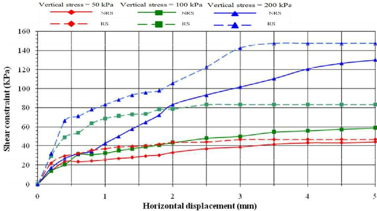
**Figure 1.** Constraint/deformation curves of the sand under different normal efforts (with or without fibre inclusion at 0.5% of the sand weight, FL= 0.5 cm).
