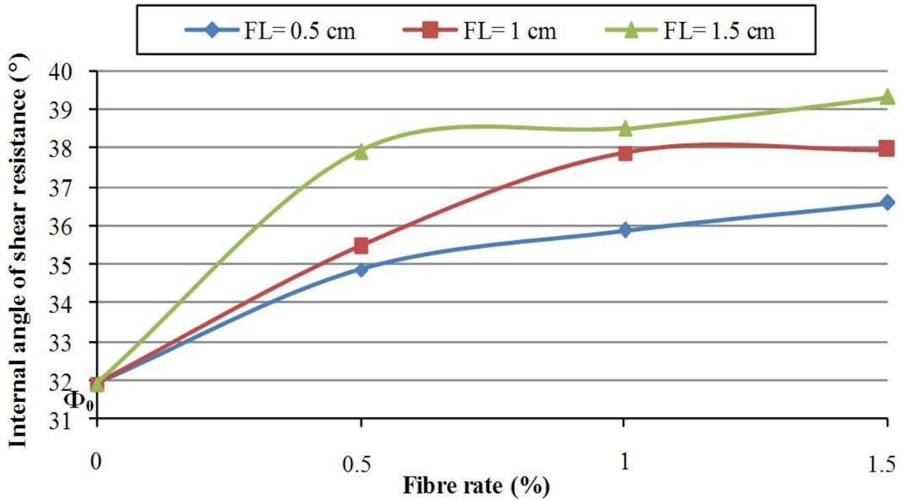
**Figure 10.** Variation of shearing strength angle of sand according to the rates of included PP fibre different lengths.  $\Phi_0$ : Friction angle of non-reinforced sand ( $^\circ$ ); FL: fibre length (cm) .
