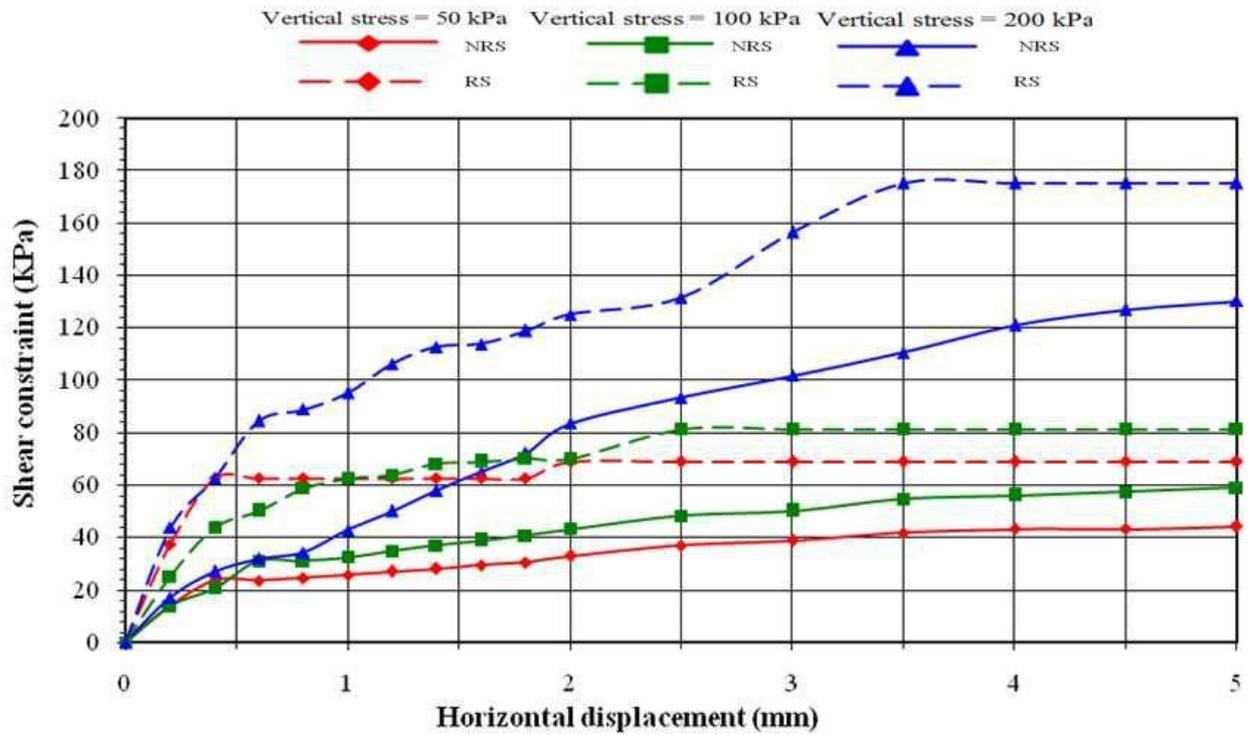
Figure 8. Constraint/deformation curves of the sand under different normal efforts (with or without fibre inclusion at 1.5% of the sand weight, FL=1 cm).
