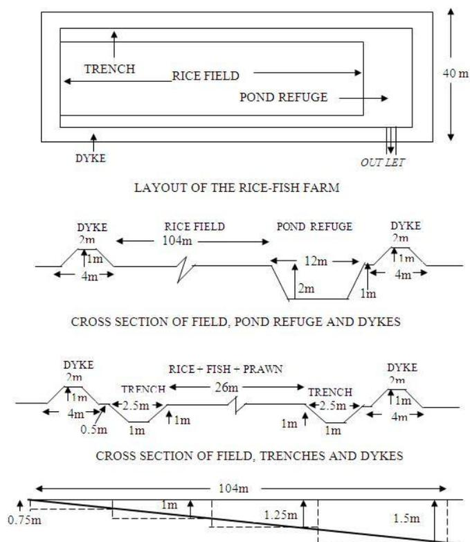
**Figure 2.** Design of the rainfed lowland rice-fish based integrated farming system at RRLRRs, Gerua (0.5 ha).
