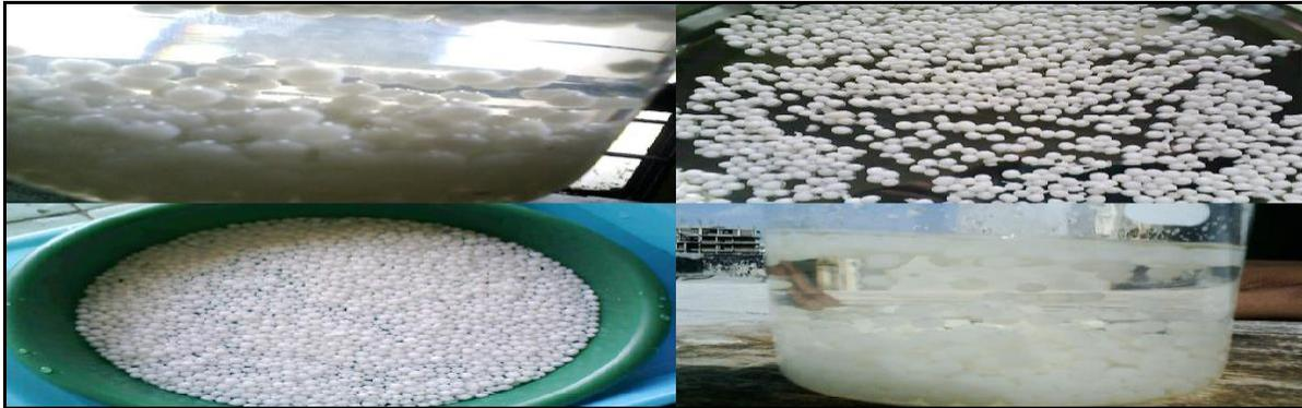
**Figure 2.** Particle size development of chitosan- doped metal bio-composite bid.
