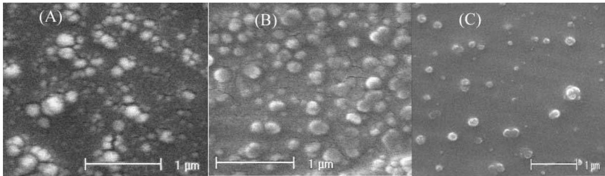
**Figure 3.** SEM images of CR NPs of PCLF530 (A), CR NPs of PCLF1250 (B) and CR NPs of PCLF2000 (C) (NP formulation 1, 2 and 3 respectively, Table 5). CR, Crosslinked.
