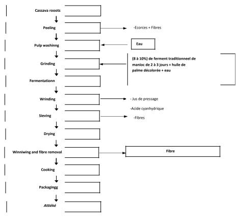
Figure 1: Process of attieke production in Côte d'Ivoire
