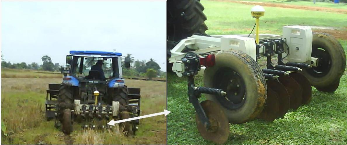
**Figure 3.** The veris 3100 sensor showing GPS receiver and six coulters to determine electrical resistance across the soil profile.
