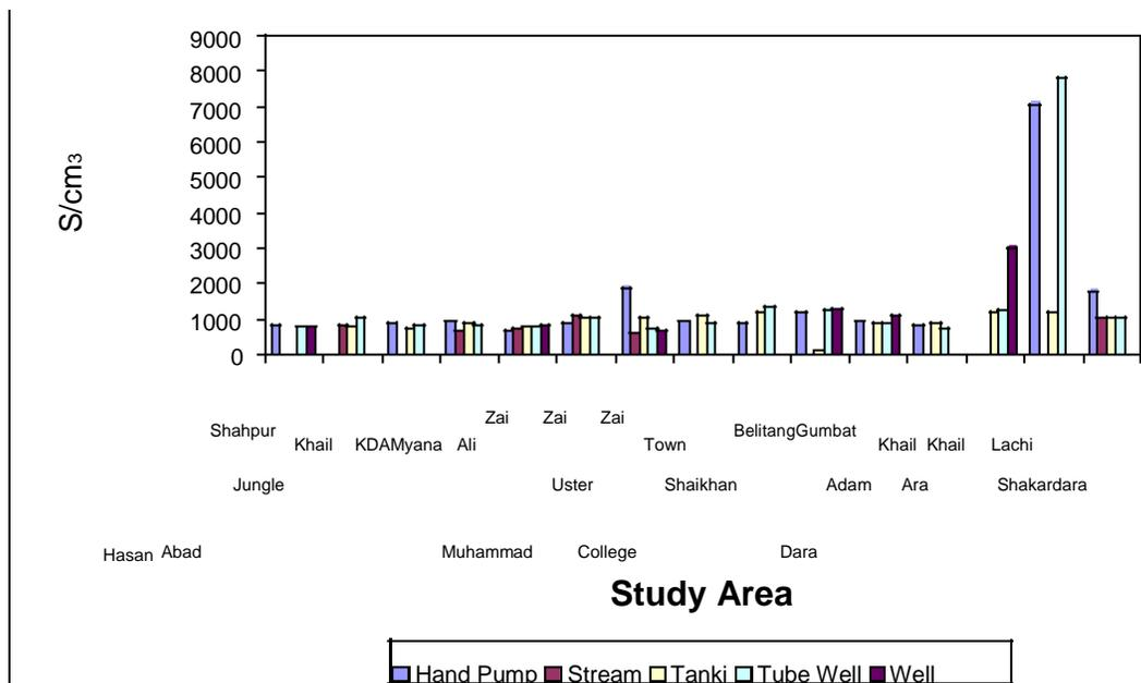
Figure 3. Electrical conductance of water samples.
