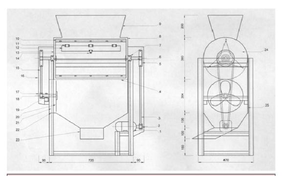
Weight: 90 kg; Overall size =  $900 \times 470 \times 1270$  mm; Power Drive: 0.75 hp petrol or diesel engine. Application Potential: For threshing Cowpea and on replacement of beater belts rice, soybeans, sorghum, millet, groundnuts and maize; Advantages: Compact design for easy operation and easy maintenance, highly portable, grain collection feature minimizes spillage, easy collection of biomass and minimum breakage; Status: Research and development stage
