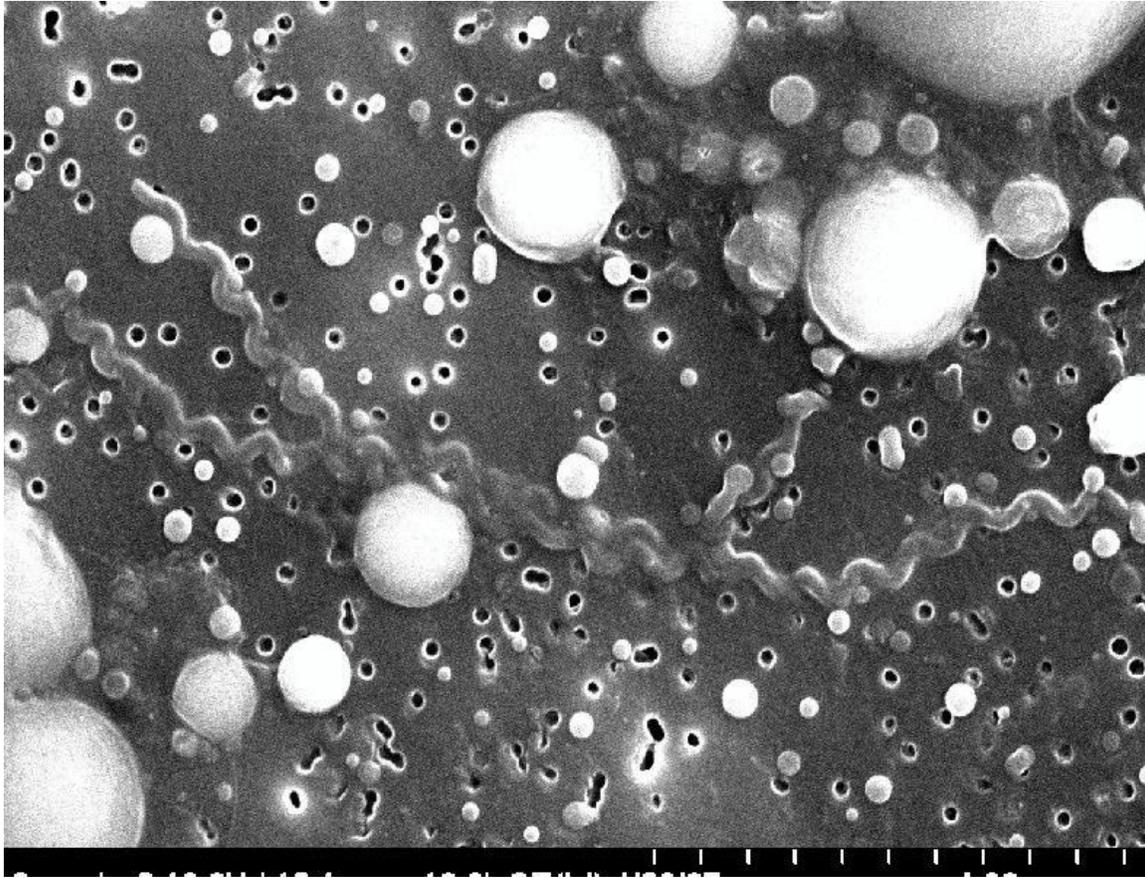
**Figure 4.** *Leptospira* spirochetes on the surface of a 0.22-  $\mu$ m pore diameter filter (Durapore Polyvinylidene fluoride membrane). Surface of filter indicate overlapping pores that could be large enough to allow passage of leptospires under vacuum (Bar, 4.0  $\mu$ m).
