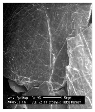
Figure 2. SEM analysis of chitin before adsorption of dye.
