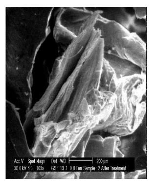
Figure 3. SEM analysis of chitin after adsorption of dye.
