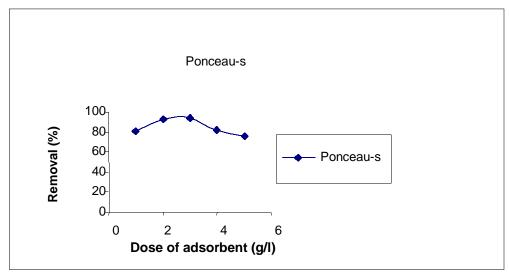
**Figure 8.** Effect of dose of adsorbent on the removal of dye at normal P<sup>H</sup> and contact time=120 min and concentration of dye is 50 ppm.
