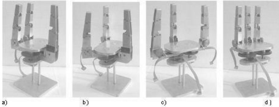
**Figure 4.** The proposed hand prototype with different finger positions: a) Fingers 2 and 3 opposite with finger 1; b) three fingers centripetal; c) fingers 2 and 3 parallel, finger 1 is free; d) three fingers parallel in one side.
