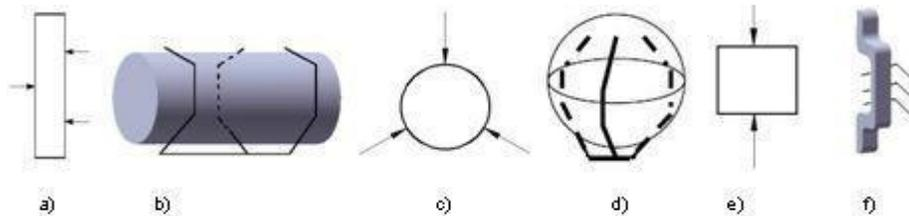
**Figure 5.** Grasp configurations: a) three fingers parallel pinch; b) three fingers cylindrical envelop; c) three fingers centripetal pinch; d) three fingers centripetal envelop; e) two fingers parallel pinch; f) three fingers parallel pull.
