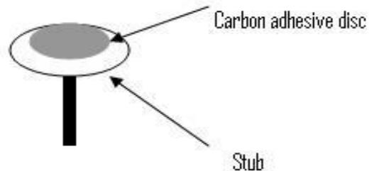
**Figure 2.** Environmental scanning electron microscope stub.
