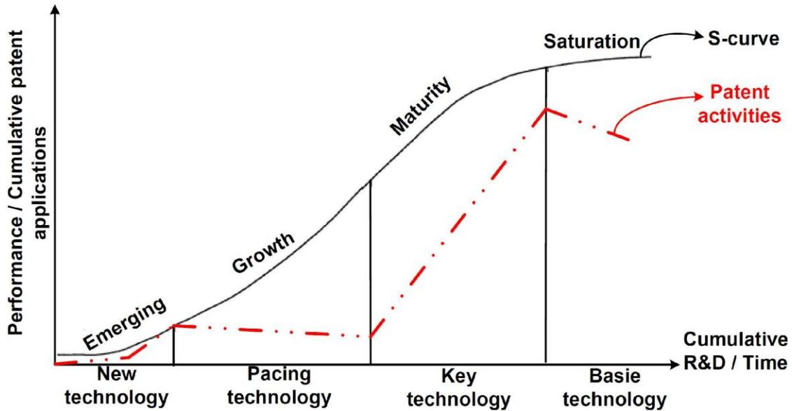
Figure 1. Scheme of integration for technological S-curve and patent activities.
