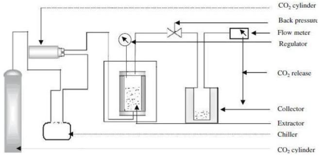
Figure 1. Supercritical CO<sub>2</sub> apparatus (Pradhan et al., 2010).
