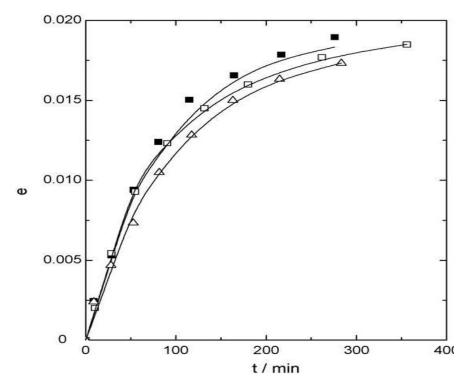
**Figure 3B.** Influence of plant mean particle diameter in the supercritical extraction of sage oil, e vs t (min), experiments 90 bar-40°C-1.32 kg/h-0.8mm, ; 90 bar-40°C-1.32 kg/h-0.5 mm, ; 90 bar-40°C-1.32 kg/h-0.3 mm, ; — Sovová's model (Langa et al., 2009)
