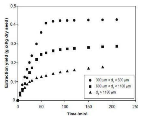
**Figure 3A.** Effect of particle size on the extraction yield of sesame oil with time at 50°C, 350 bar and 1.81 g CO<sub>2</sub>/min (Dökeret al., 2010).
