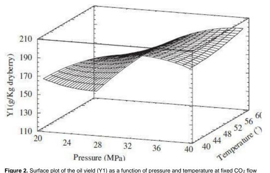
**Figure 2.** Surface plot of the oil yield (Y1) as a function of pressure and temperature at fixed CO<sub>2</sub> flow rate of 15 L/h and extraction time of 60 min (Xu et al., 2008).
