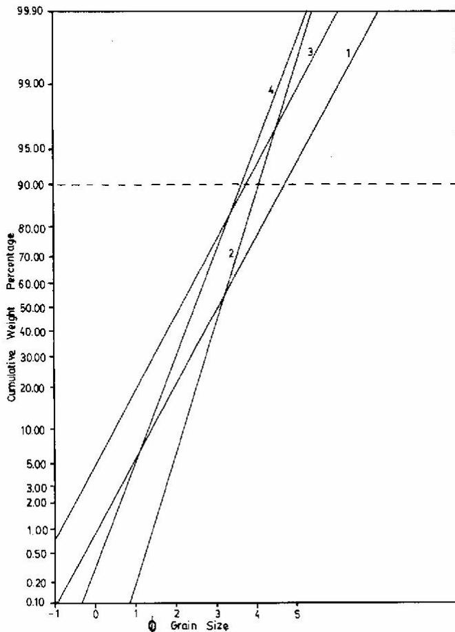
**Figure 7.** Probability plot based on results of sieve analysis of samples. Note position of  $d_{10}$  of samples.
