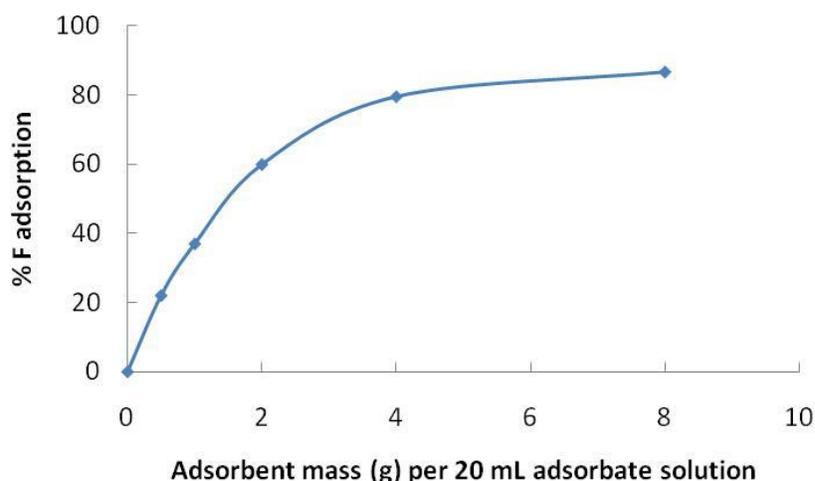
**Figure 3.** Effect of change in mass of LM-1 on its adsorption of F from 1000 mg/L F solution at 297 K.
