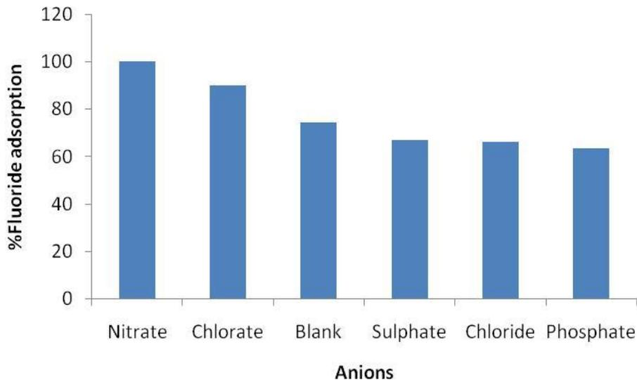
**Figure 6.** Effect of different anions on adsorption of F onto LM-1 from a 1000 mg/L F solution at 2 g per 10 mL adsorbent dosage and 297 K.
