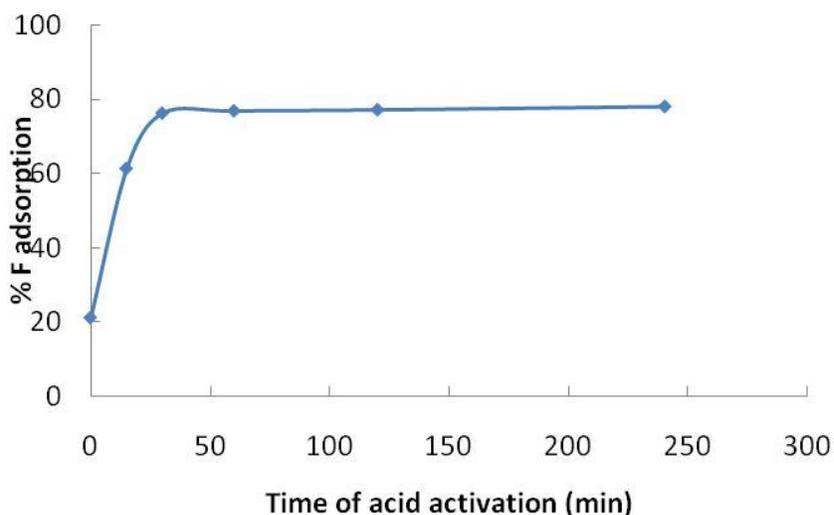
**Figure 2.** Effect of acid activation on LM-1 adsorption of F from 1000 mg/L F solution using 2 g per 10 mL adsorbent dosage at 297 K.
