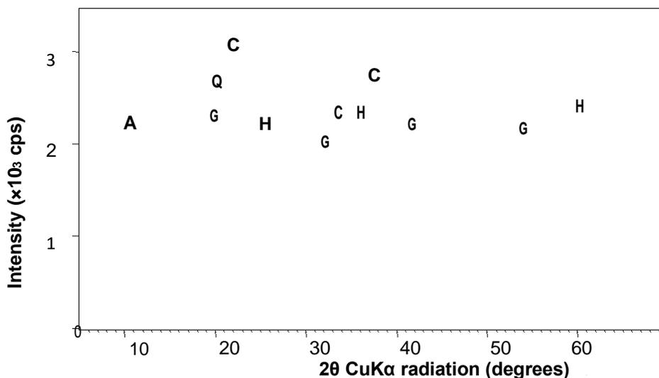
**Figure 1.** XRD pattern of Lateritic mineral adsorbent material (LM-1), Q=Quartz, C=Cristobalite, G= Goehite, H = Haematite, A = Contribution from Amorphous matrix.
