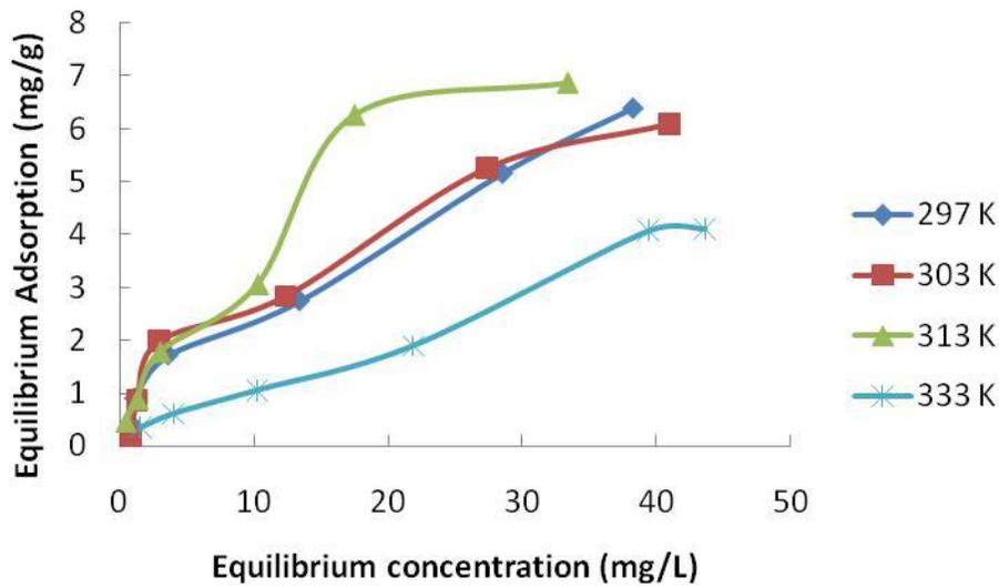
**Figure 7.** Adsorption isotherms for F uptake by LM-1 from 1000 mg/L F solution at pH 3.32 using 0.2 g/mL adsorbent dosage and 297 -333 K.
