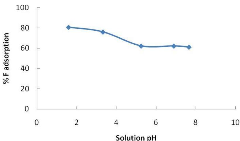
**Figure 4.** Effect of solution pH on F adsorption onto LM-1 from 1000 mg/L F solution using 2 g per 10 mL adsorbent dosage at 297 K.
