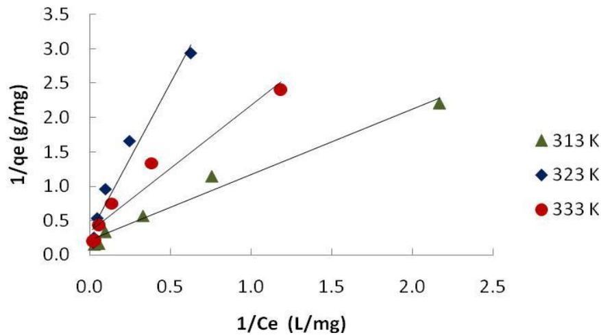
**Figure 8.** Langmuir adsorption isotherms for F adsorption onto LM-1 at 313 K, 323 K and 333 K.
