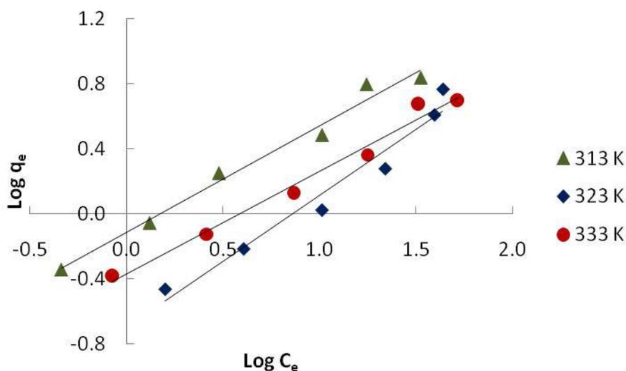
**Figures 9.** Freundlich adsorption isotherms for F adsorption onto LM-1 at 313 K, 323 K and 333 K.
