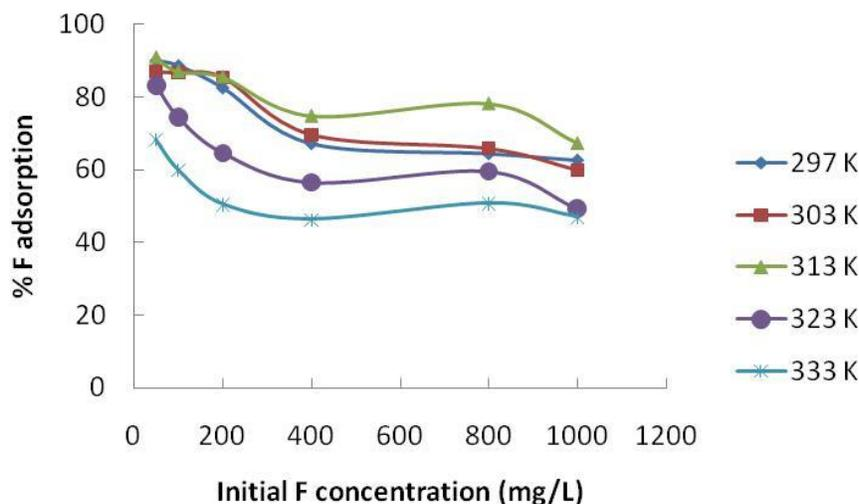
**Figure 5.** Effect of solution temperature on LM-1 uptake from 1000 mg/L F solution using 2 g per 10 mL solution.
