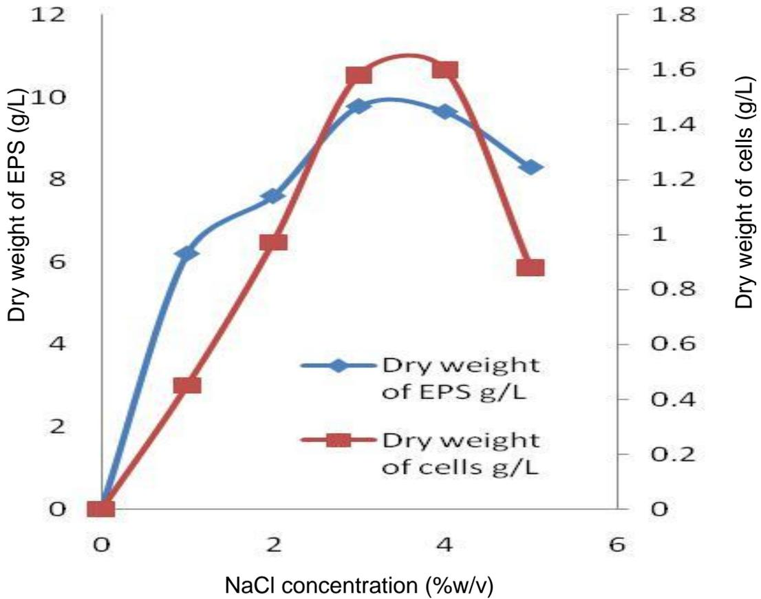
**Figure 5.** Effect of Different concentrations of NaCl on the production of EPS by *Ps eu doal t er omo nas* sp. AM. Results are average of three replicate flasks per experiment.
