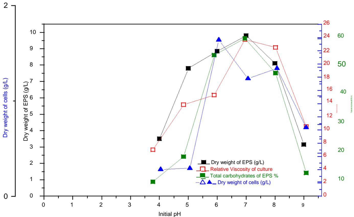
**Figure 3.** Effect of Initial pH on the production of EPS by *Ps eu doal t er omo nas* sp. AM. Results are average of three replicate flasks per experiment.
