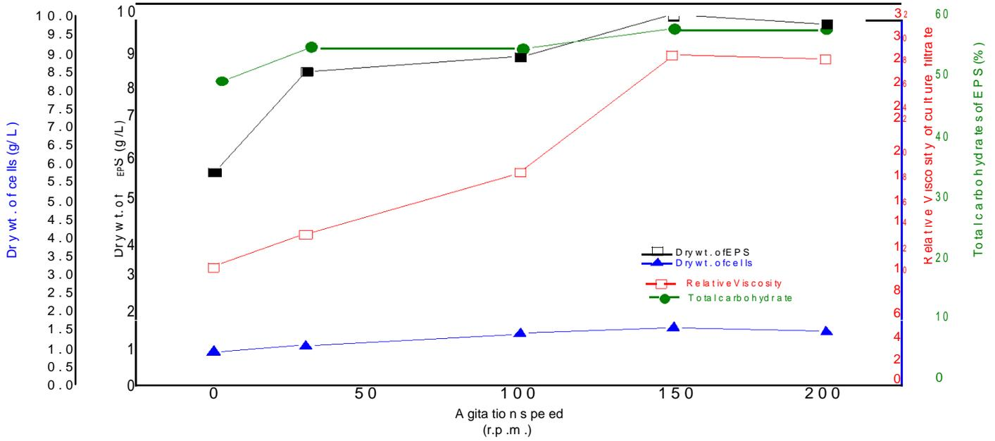
**Figure 4.** Effect of agitation speed on EPS production by *Ps eu doal t er omo nas* sp. AM. Results are average of three replicate flasks per experiment.
