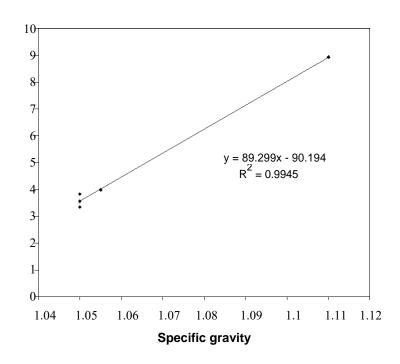
Figure 4. Correlation between reducing sugar contents and specific gravity of fermented sugar syrup.
