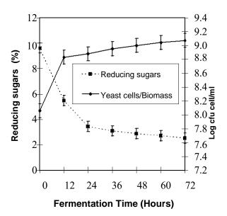
**Figure 5.** Changes in reducing sugar contents and biomass associated with fermentation of sugar syrup with time.
