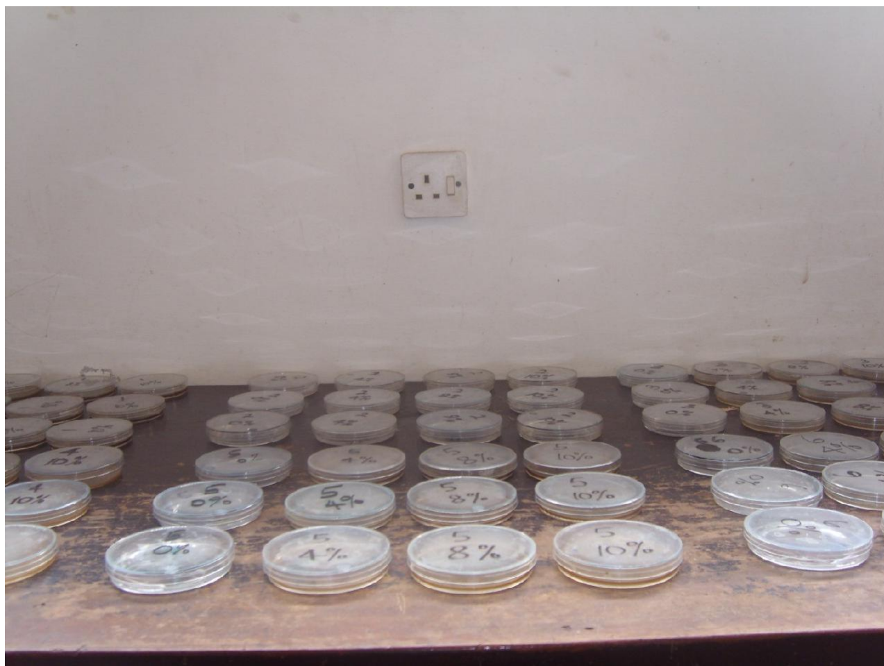
Figure 1. Set up of aqueous extracts of organic waste compounds. Cold aqueous extracts (compost, poultry manure, cocoa bean testa, citrus waste, palm bunch waste and distilled water-control). Four concentration levels of extracts (0%-distilled water, 4, 8 and 10%).
