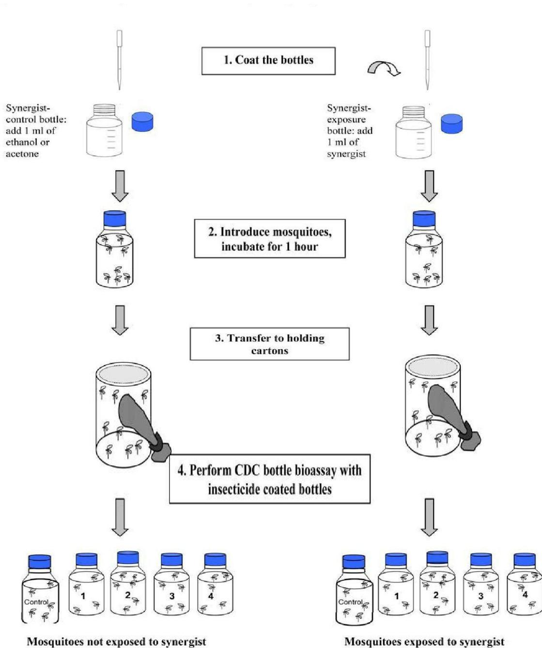
**Figure 2.** Diagram for performing the CDC bottle bioassay with synergists [CDC: Methods in *Anopheles* Research, 2010].
