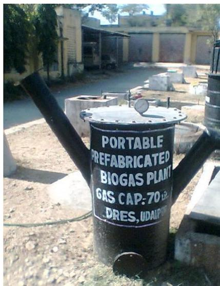
**Figure 2.** Prefabricated plant for laboratory study.
