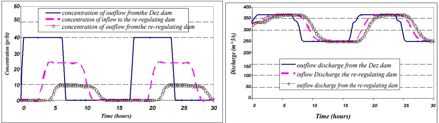
Figure 3. Hydrograph of flow and sediment concentration of the Dez River for the option G2-40 30 based on the model results.
